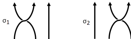
Figure 2.2: \sigma_1 : the operation of interchanging the particles at 1 & 2 by moving 1 counter-clockwise around 2. \sigma_2 : the operation of interchanging particles 2 & 3 by moving 2 counter-clockwise around 3
